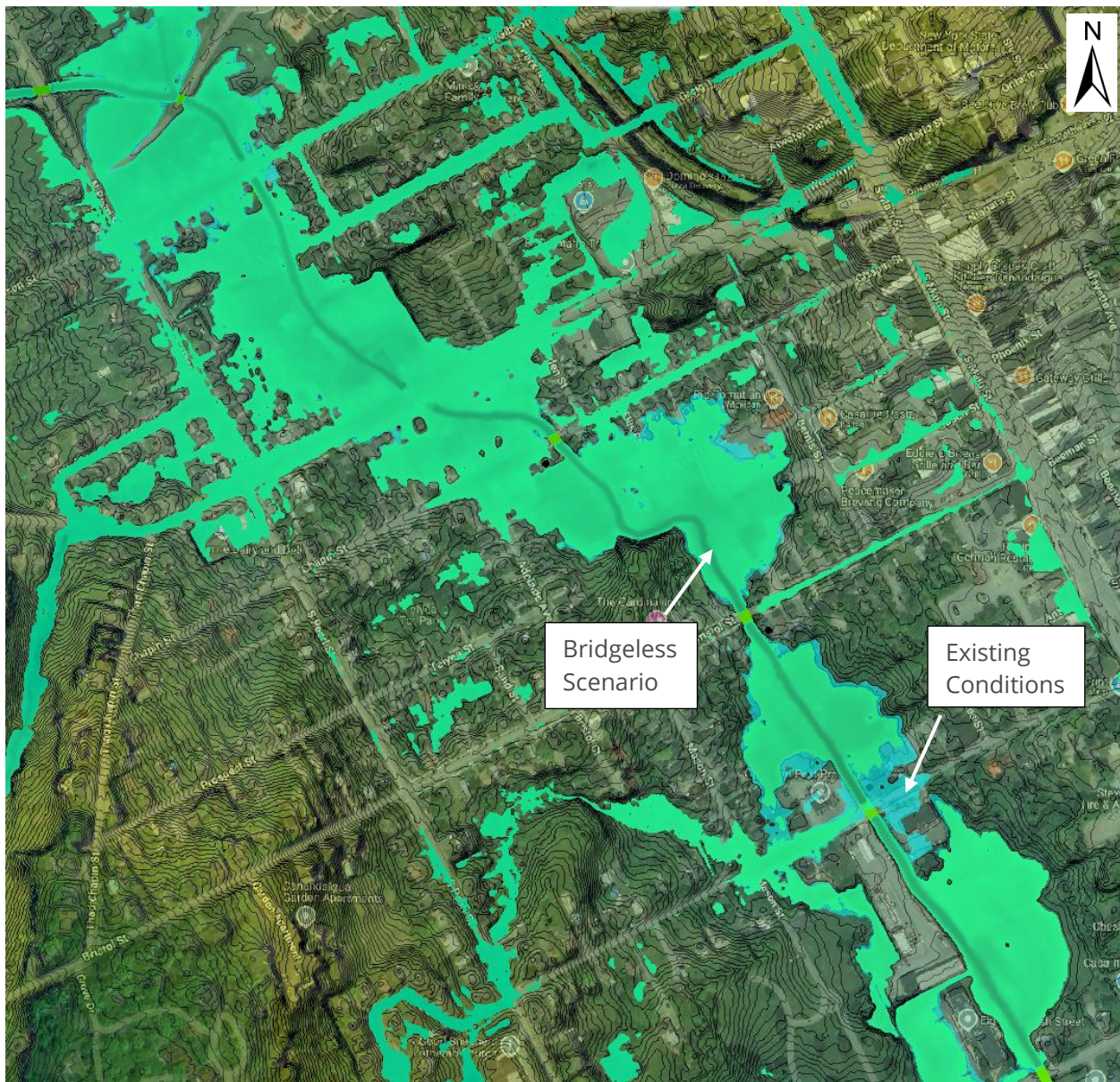
Figure 8: Comparison of 100-year inundation area with and without bridges
