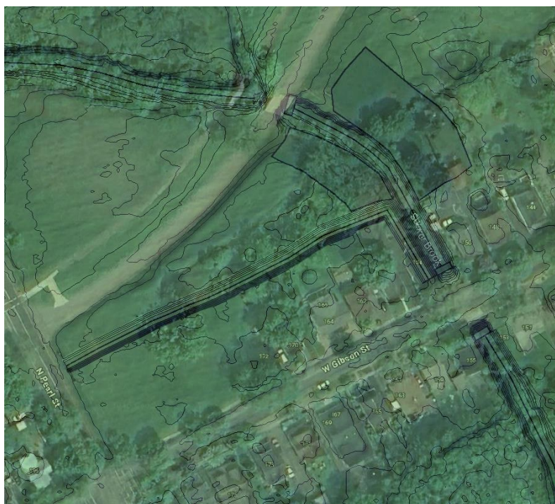
Figure 14: Alternative 3 proposed conditions, showing berm and floodplain benches
